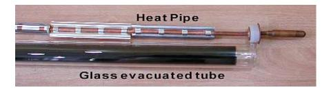
The heat pipe transfers the heat to the manifold by a very simple method. The copper heat pipe is hollow and contains a small amount of fluid. The hollow centre of the heat pipe is a vacuum, so that at even at temperatures of around 40°C the fluid will vaporize (boil). The vapor rises to the tip (condenser) of the heat pipe where the heat is transferred to the water flowing through the
