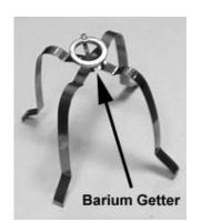
The Getter is located at the bottom of the outer tube.
