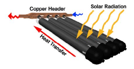
The heat pipe is a very efficient means of transferring heat from within the evacuated tube to the water. The following diagram shows both the glass evacuated tubes and the copper heat pipe. The heat pipe is simply inserted into the glass tube, held in place with high quality silicon based glue.
