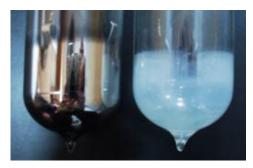
Left Tube = Good --- Right Tube = Faulty In the left tube two "arms" of the getter are visible. The right tube has had the inner tube and getter removed.
