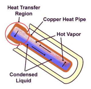
This method of heat transfer is thousands of times more efficient than a solid copper rod. Heat is therefore very efficiently transferred from the glass evacuated tube to the water. Since no water is flowing through the collector tubes and the tubes are hermetically sealed it does not suffer from corrosion problems as is the case with other solar collector types.
