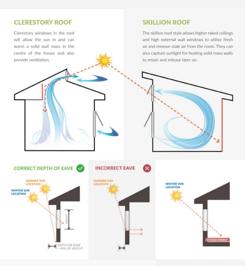
Eave overhang will determine the amount of natural sunlight and energy to enter a room. An eave that does not have enough overhang depth will let too much sunlight in during Summer. An increased eave overhang will prevent the home from warming as the sun is unable to reach the external wall mass.
